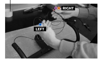
The Grey connector must exit form the central hole, passing through the stem.
