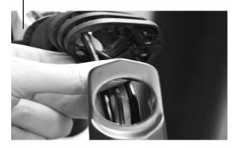
The front brake hose passes throught the head tube.
